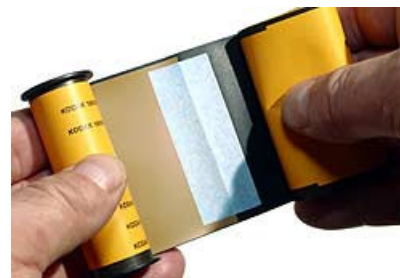
This illustrates that the film is taped to the paper. This will be important later. Continue unrolling. >>>>>>
